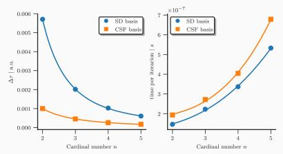
Time-step  $\Delta \tau$  (left) and time per iteration (right) vs. cardinal number of cc-pVnZ basis set for N<sub>2</sub> at  $r = 4.2 a_0$
